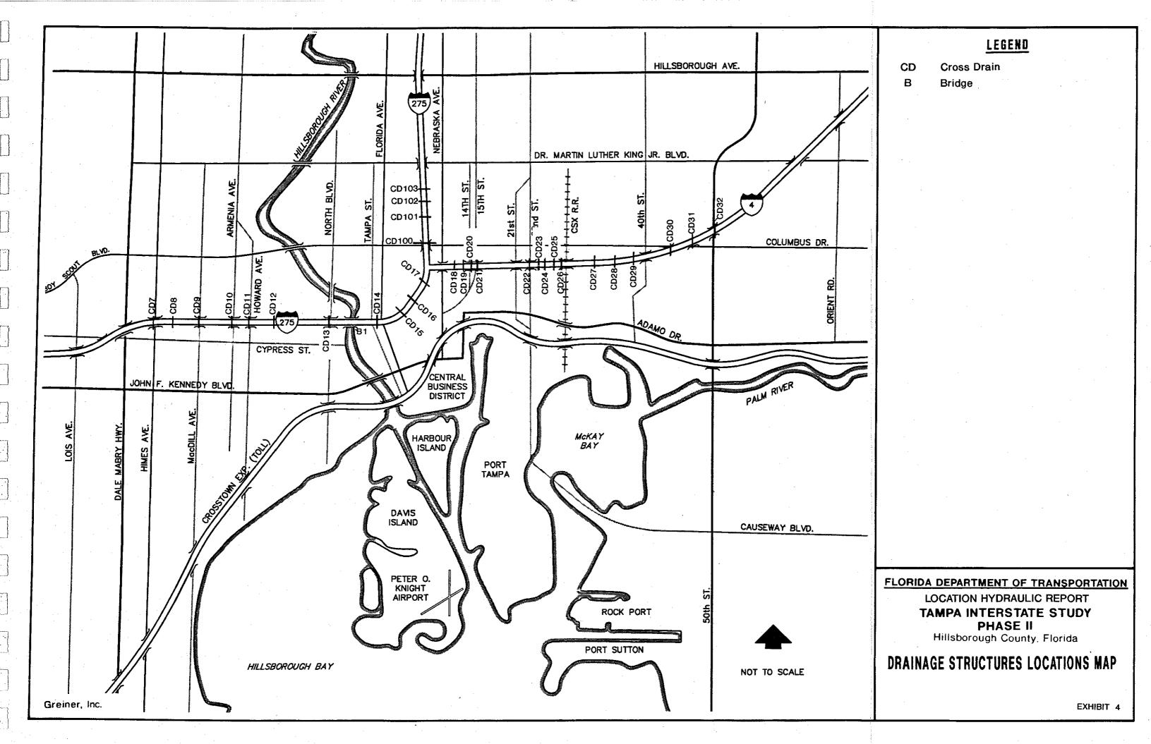
structures include 23 reinforced concrete pipes (RCP), with sizes ranging from 18 inches to 84 inches and 7 concrete box culverts (CBC), with sizes ranging from 3' x 3' to 10' x 6'.
