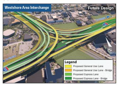
Local street improvements to enhance mobility would include the reconnection of Reo Street, Occident Street, and Trask Street under I-275 providing additional north-south connectivity. A new on-ramp from Reo Street to southbound I-275 would provide direct express lane access. A diverging diamond interchange at Reo Street will provide new connections between Kennedy Boulevard and Cypress Street.
